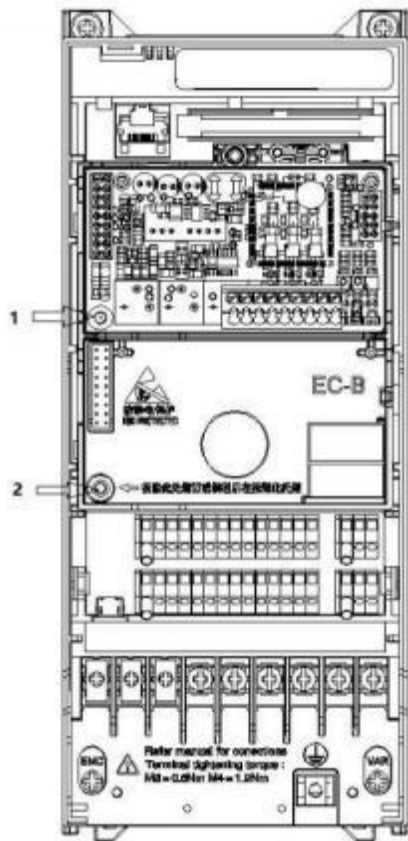
Fig. 9-5 Installation diagram of PG card
